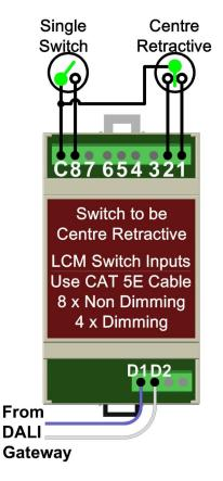
Wiring -when not supplied as part of a panel.
